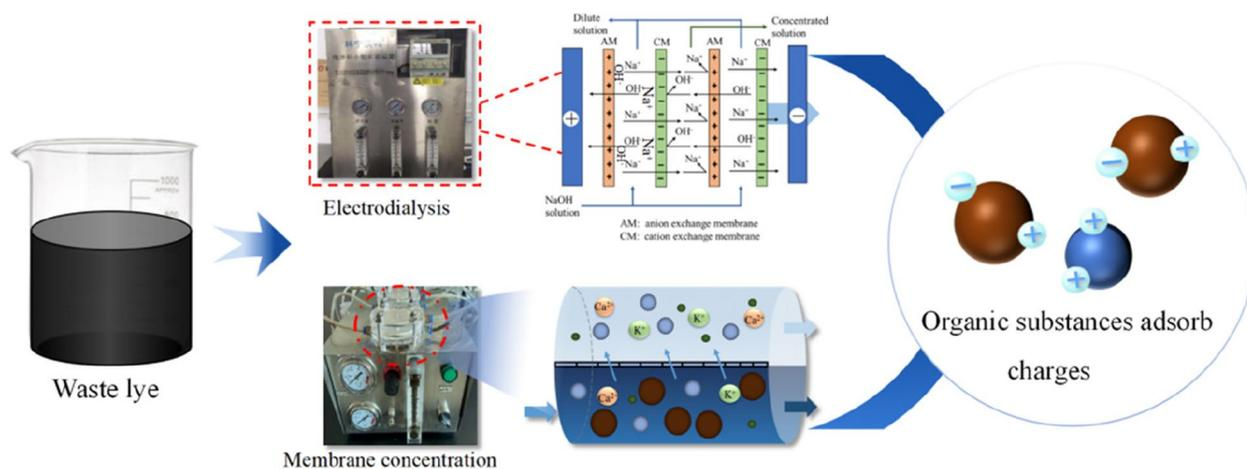
**Fig. 4** Speculating the mechanism of charge affecting the electrodialysis membrane and membrane concentration process
