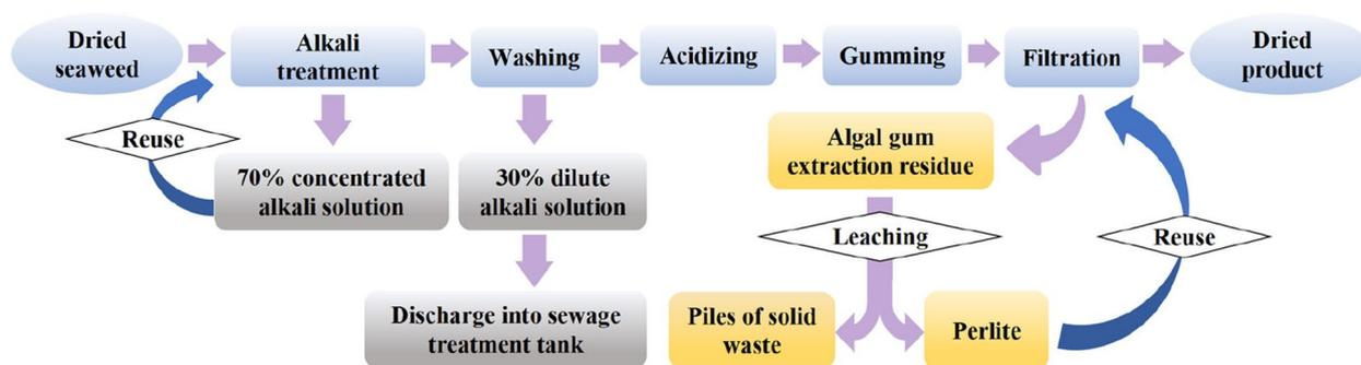
**Fig. 1** Flow chart of the seaweed gel extraction process
