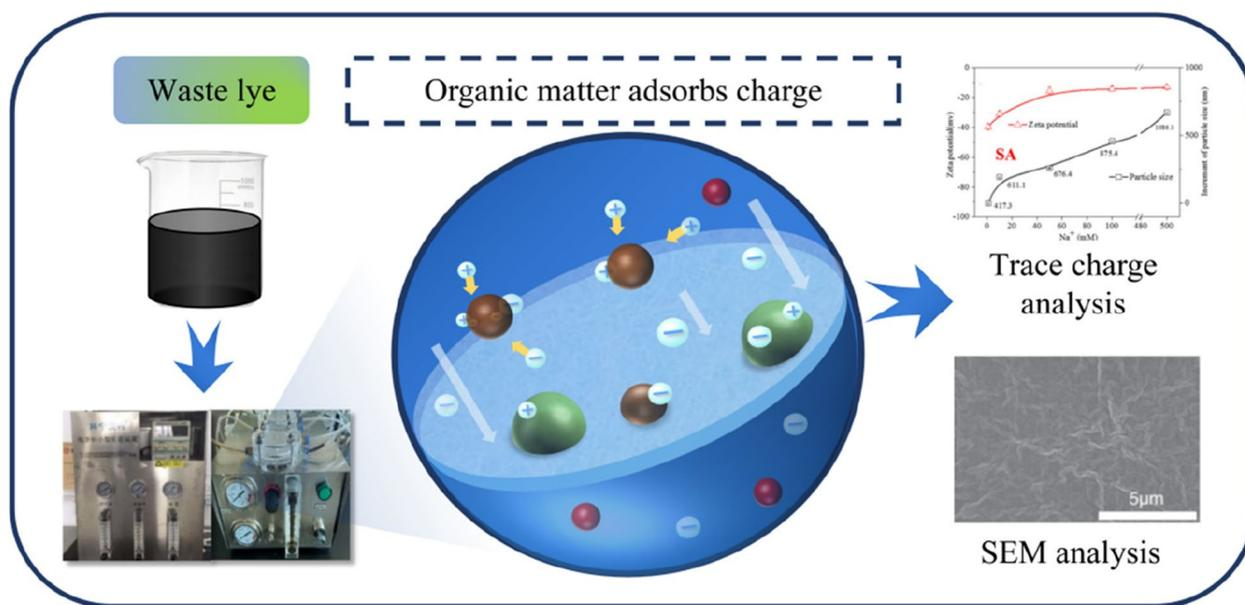
**Fig. 6** Study on the mechanism of the adsorption of organic matter from waste lye during seaweed gel extraction
