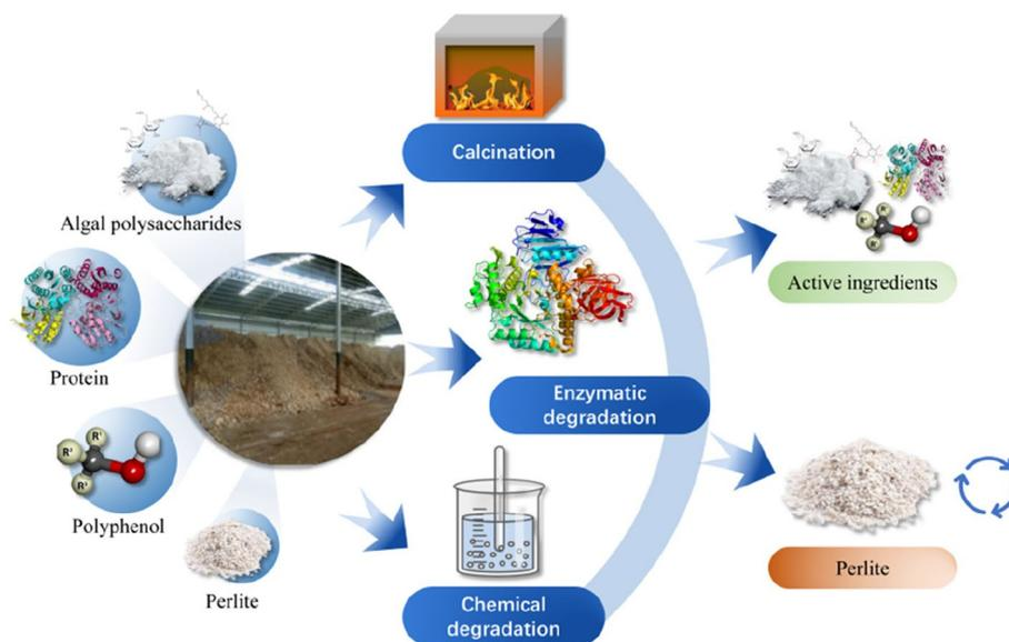
**Fig. 3** The treatment technologies for solid waste residue from seaweed gel extraction
